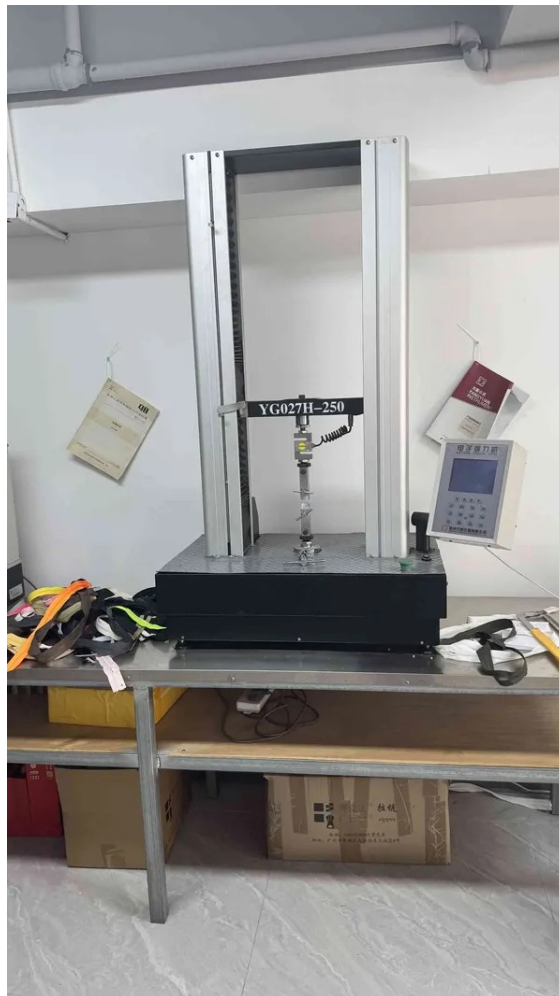
QC tensile testing equipment used to check zipper pull force and assembled strength.
